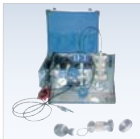
Nutsche test equipment (Filtration area: 0.001m 2 )
